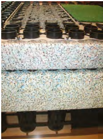
This mockup shows a typical cross section of engineered subsurface that contributes to permeable surfaces. Source: O'Brien360
