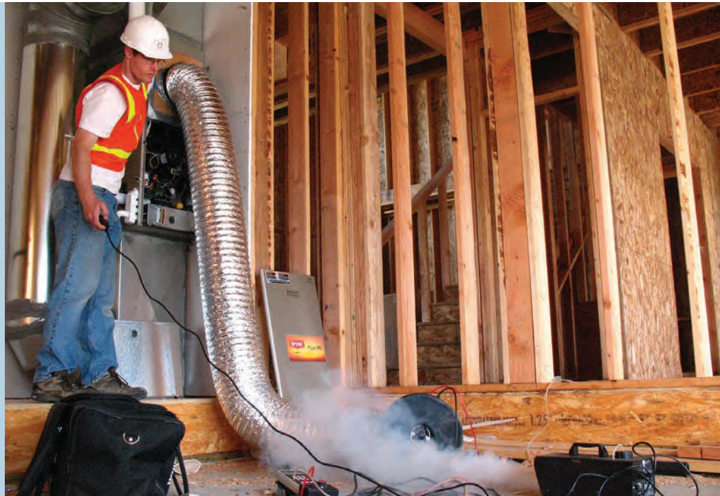
Duct leakage testing in a new home. Non-toxic smoke can be used to locate leakage areas, especially during framing in new construction. Source: O'Brien360
